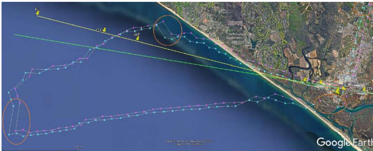
Figure 1: Lateral Flight Profile based on radar data (in Google Earth projection) (Magenta: Original radar track; Cyan: Corrected radar track)
