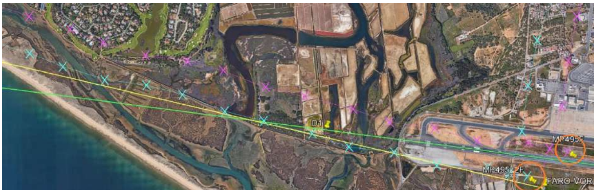
Figure 3: Lateral Flight Profile based on radar data (final segment, zoomed in Google Earth projection) (Magenta: Original radar track; Cyan: Corrected radar track)
