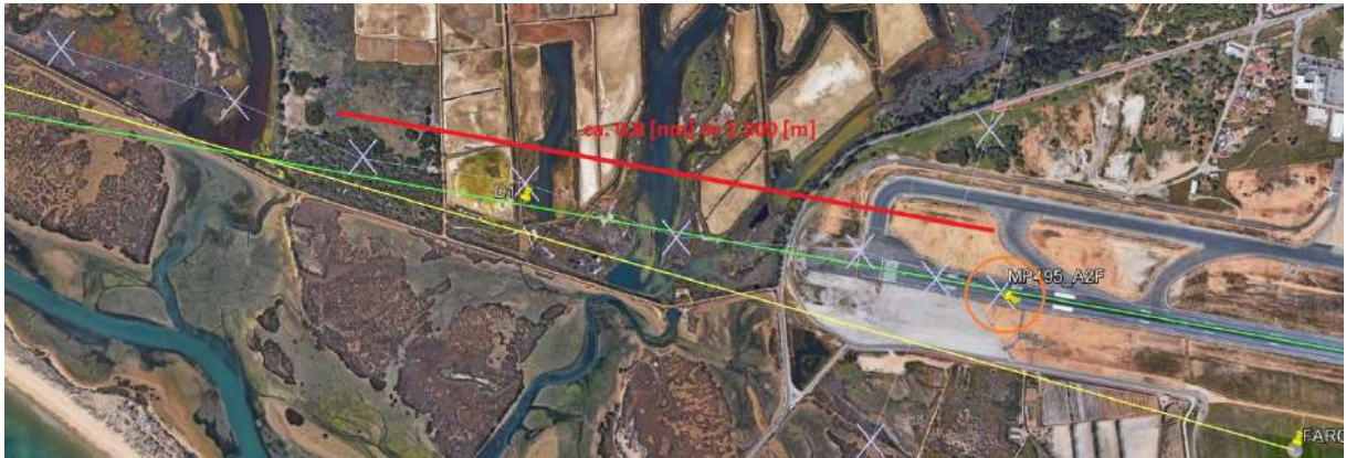
Figure 7: Lateral Flight Profile based on radar data (final segment, zoomed in Google Earth projection) (Purple: Shifted to touchdown point corrected radar track)
