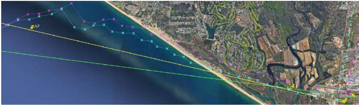
Figure 2: Lateral Flight Profile based on radar data (from IAF to touchdown, zoomed in Google Earth projection) (Magenta: Original radar track; Cyan: Corrected radar track)
