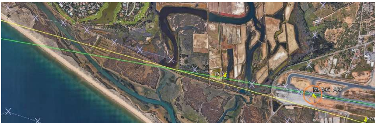
Figure 6: Lateral Flight Profile based on radar data (final segment, zoomed in Google Earth projection) (Purple: Shifted to touchdown point corrected radar track)
