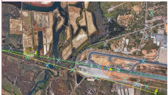
Figure 5: Lateral Flight Profile based on radar data (final segment, zoomed in Google Earth projection) (Purple: Shifted to touchdown point corrected radar track)
